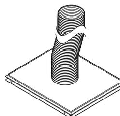
**3869600—Exhaust Connection Kit.** For connection to house exhaust or other exhaust system. Includes powder-coated steel connector with 5.0" dia. collar, 14.0" of 5.0" dia. flexible duct, and two clamps. **Requires user-supplied exhaust system capable of exhausting 150 CFM (4.2 m3/min) at a vacuum of 0.5 inch of water (125 Pa).** Shipping weight 10 lbs. (5 kg)
